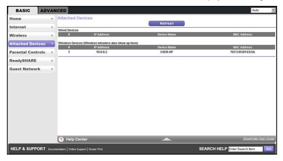
Wired devices are connected to the wireless modem router with Ethernet cables. Wireless devices have joined the wireless network.
